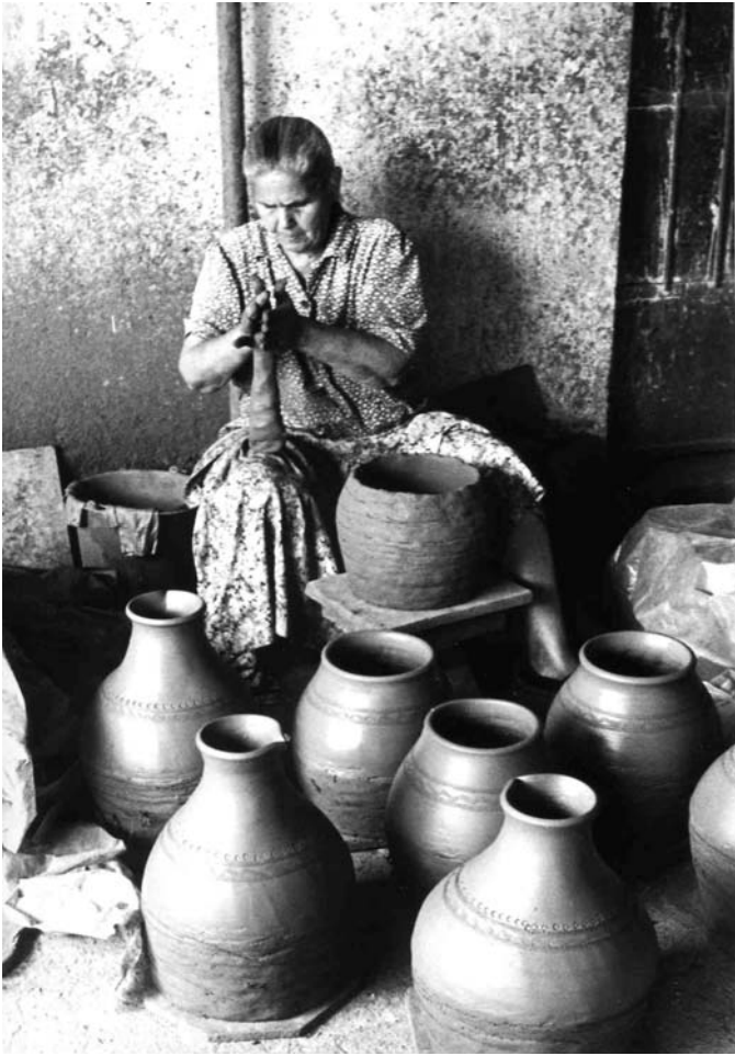
Fig. 8-3. In Kornos, all potters finish stage one of manufacture by decorating the shoulder prior to handle application. The order of work in the two mountain communities is opposite, and only after handle attachment is the decoration carefully organized. Here, a Kornos potter rolls a coil in the air for a cooking pot during stage one of manufacture. After shaping the rim, the shoulder is smoothed and decorated. In stage two, the handles smudge part of the incised pattern on cooking pots and jugs (with pinched spouts) that dry in the foreground. At an even later stage, the strings supporting the thick lower body are removed and a rounded bottom is cut from the flat base. Photo by author.
